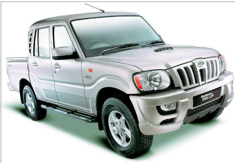
TAKE-AWAY INDIAN: The Pik-Up range consists of single and dual-cab utes and cab-chassis models, with two or four-wheel drive. All boast a payload of at least a tonne
