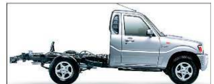
TAKE-AWAY INDIAN: The Pik-Up range consists of single and dual-cab utes and cab-chassis models, with two or four-wheel drive. All boast a payload of at least a tonne
